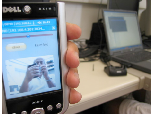
Figure 2: EyesWeb Mobile running on a DELL Axim X51. Images are captured by a webcam on the notebook on the background and streamed to the mobile via a standard WLAN connection.
