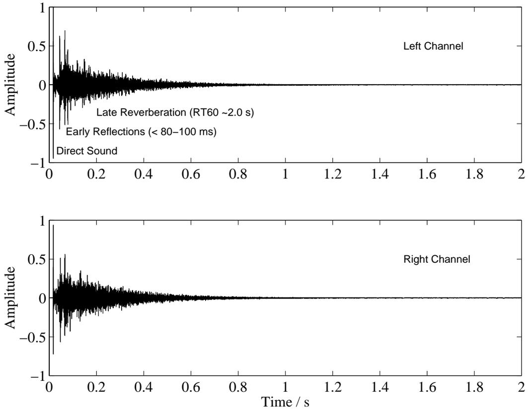
Figure 2.4: A binaural room impulse response measured in a concert hall. The room impulse response can be divided into the direct sound, early reflections, and late reverberation.
