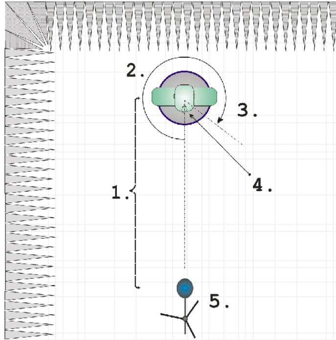
Figure 3.5: Measurement installation in the anechoic chamber during reciprocity method. **1.** Distance to source (spherical loudspeaker): 2 meters. **2.** Azimuth angle. **3.** Rotational direction of the BK4128 dummy head. **4.** Measurement microphone (Sennheiser KE 4-211-2) installed in the mouth of the dummy head. **5.** Spherical loudspeaker (Audax AT100M0) on stand (Huopaniemi et al., 1999a).
