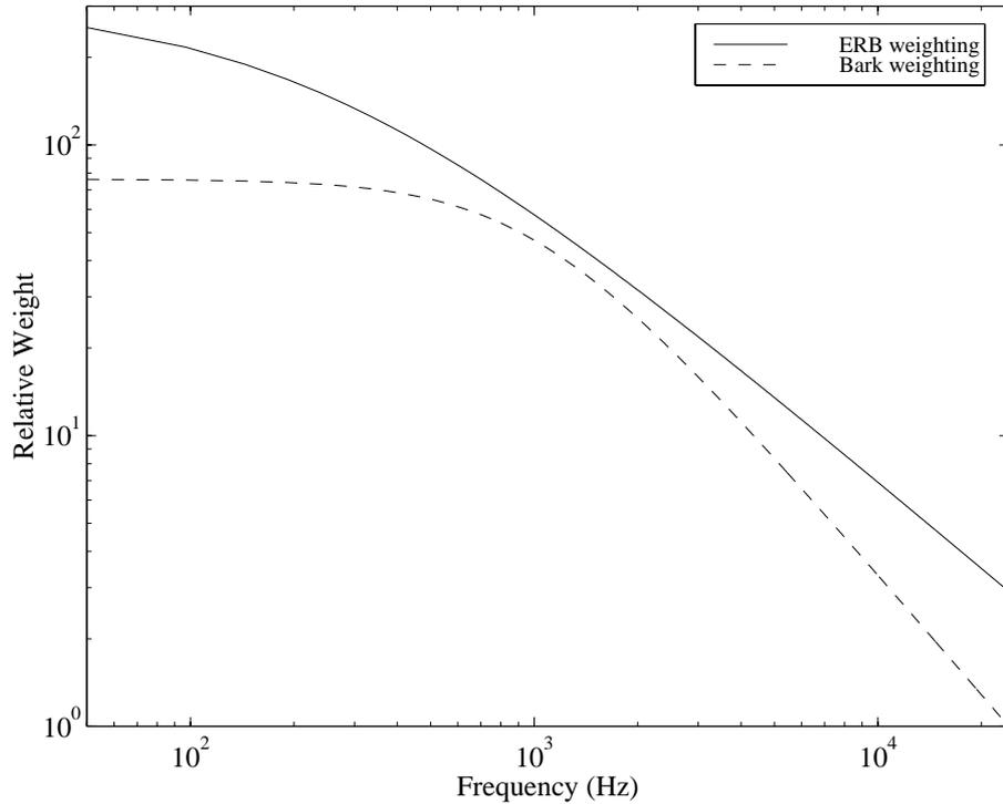
Figure 5.18: Auditory weighting functions as a function of frequency,  $f_s = 48$  kHz.
