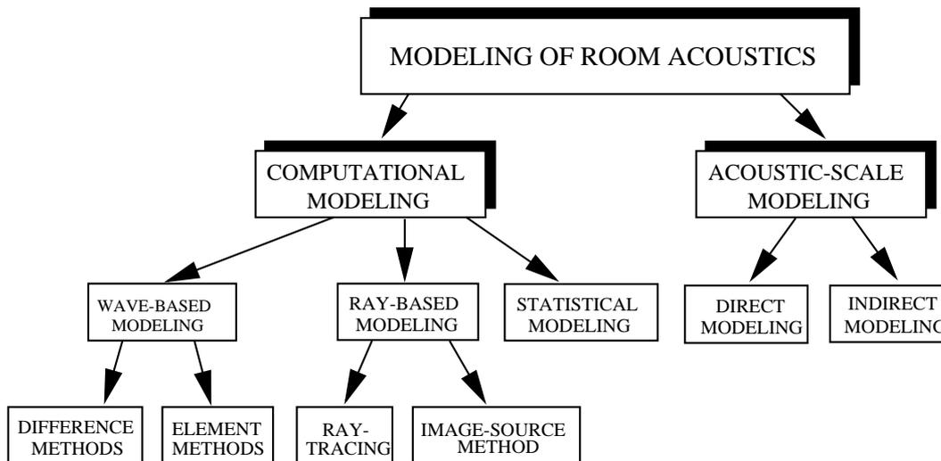
Figure 2.3: Different methods for room acoustics modeling and auralization (Savioja et al., 1999).
