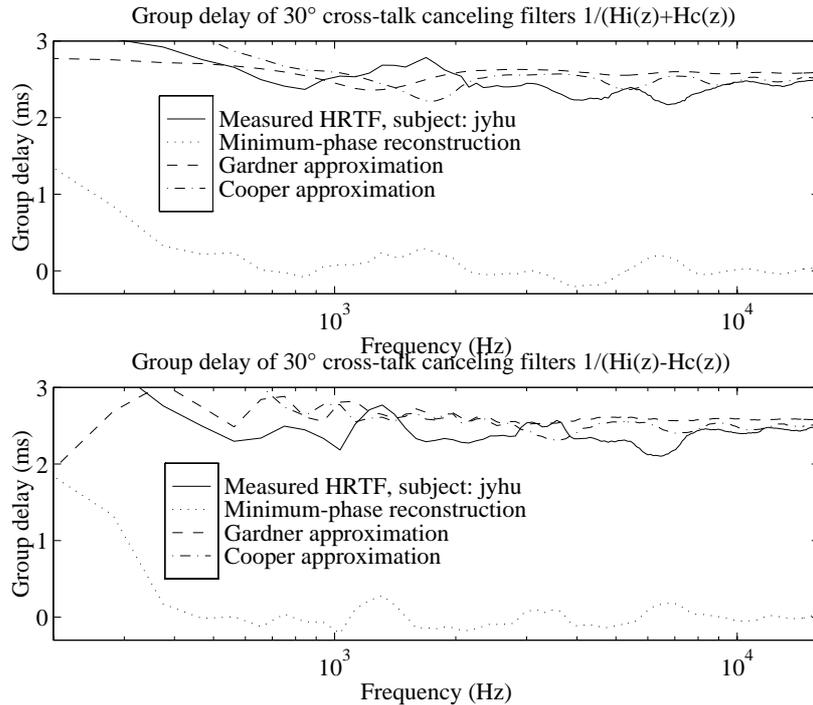
Figure 6.4: Group delay of three crosstalk canceling filters for sources at  $30^\circ$  azimuth.
