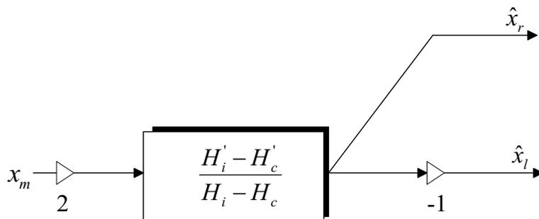
Figure 6.10: Monophonic decorrelation shuffler for synthesizing two VLs implemented with a single filter.
