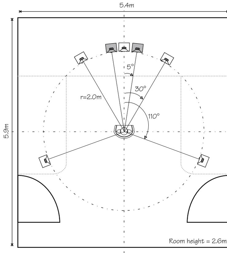
Figure 6.21: Layout of the new NRC ITU-R BS.1116-1 (ITU-R, 1997) compliant listening room and loudspeaker setup (Zacharov et al., 1999).
