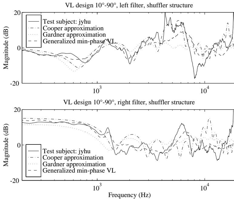
Figure 6.20: VL design magnitude responses for loudspeakers placed at  $\pm 10^\circ$  azimuth and virtual speaker placement of  $\pm 90^\circ$  azimuth. The shuffler structure was used.
