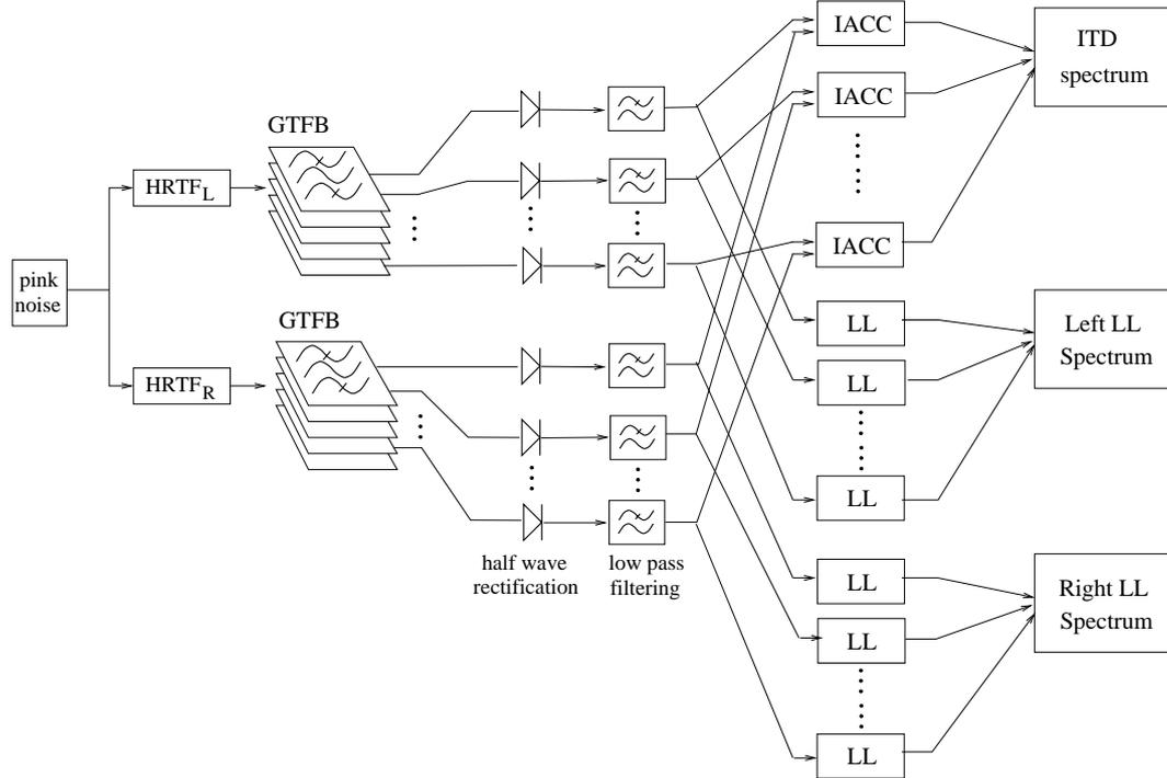
Figure 5.24: Detailed view of the binaural auditory model used in the objective evaluation of HRTF filter designs (Pulkki et al., 1999).
