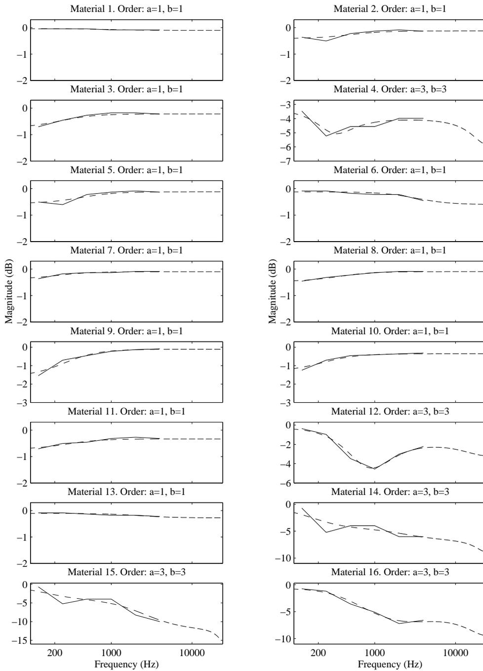
Figure 4.2: First-order and third-order minimum-phase IIR filters designed to given absorption coefficient data. Solid line: octave-band data, dashed line: IIR filter approximation.
