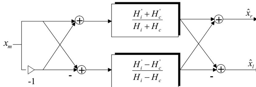
Figure 6.9: Monophonic decorrelation shuffler for synthesizing two VLs.
