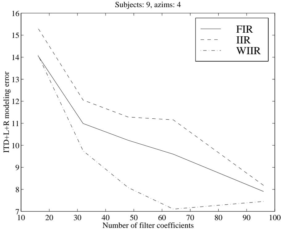
Figure 5.36: Binaural auditory model results for 9 subjects and 4 azimuth angles using three different filter design methods. The combined ITD and composite (L + R) loudness level spectrum error estimate was used (Huopaniemi et al., 1998, 1999b).
