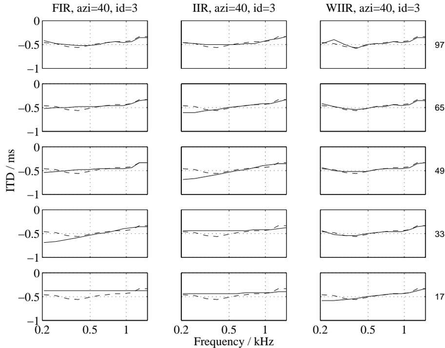
Figure 5.34: Binaural auditory model evaluation of filter design quality. ITD, azimuth angle  $40^\circ$ , person 3. Solid line: filter approximation, dashed line: reference (Huopaniemi et al., 1998, 1999b).
