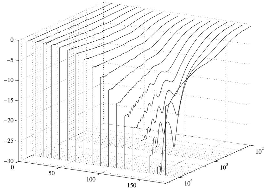
Figure 3.3: Spherical head approximation directivity at 2 meter distance. X-axis: Azimuth angle (degrees), Y-axis: Frequency (Hz), Z-axis: Magnitude (dB).
