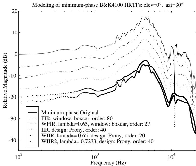
Figure 5.26: Warped filter design compared with traditional FIR and IIR designs. BK4100 dummy head HRTFs were used (Huopaniemi and Karjalainen, 1996b,a).
