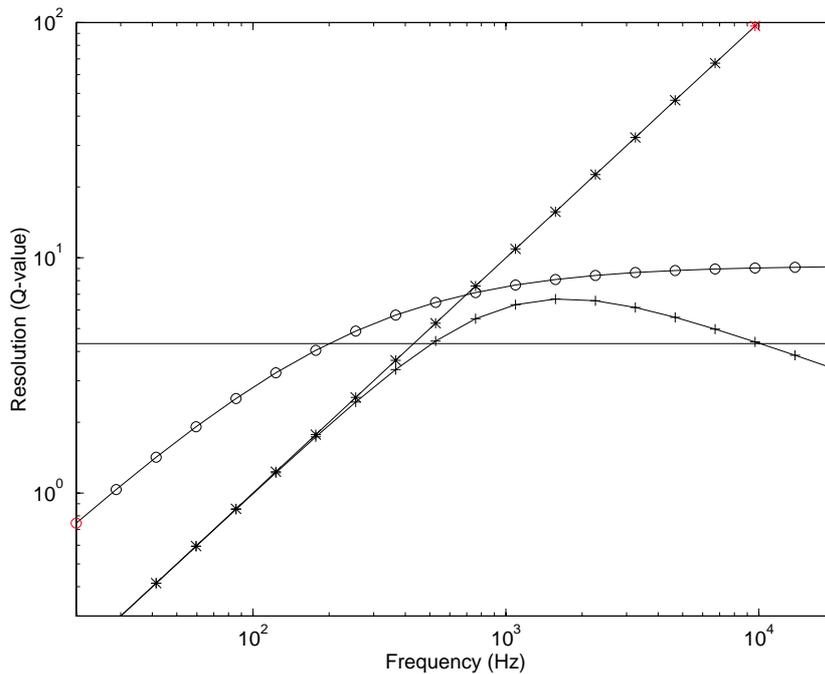
Figure 5.15: Frequency resolution (Q-value) curves as functions of frequency: Solid line = third-octave (constant Q); o-o = ERB resolution; +-+= Bark (critical band) scale; \*-\* = constant 100 Hz bandwidth (linear resolution)(Karjalainen et al., 1999).
