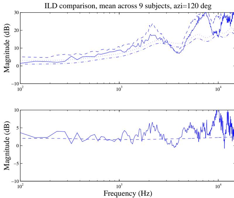
Figure 5.14: Near-field and far-field interaural level differences at  $120^\circ$ .
