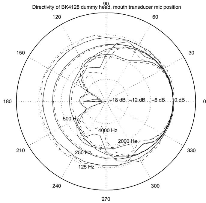
Figure 3.7: Directivity of the BK4128 dummy head using the direct method (dashed line) and the reciprocity method (solid line). The reciprocal microphone position is at the mouth opening.
