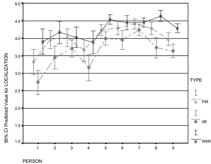
Figure 5.38: Listening test results for three filter types (FIR, IIR, WIIR). Predicted values as a function of test persons. Tested variable: localization (Huopaniemi et al., 1998, 1999b).
