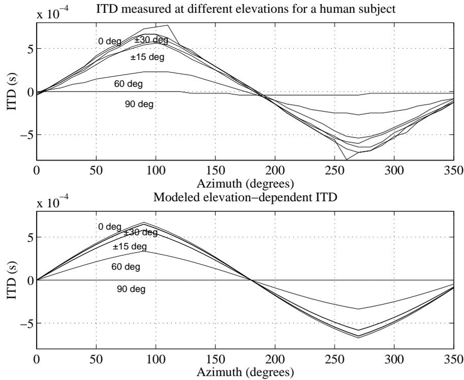
Figure 5.7: Measured and simulated ITDs at various elevation angles as a function of azimuth angle.
