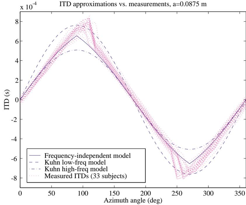
Figure 5.6: Comparison of ITD approximations to measured ITDs of 33 human subjects at  $0^\circ$  elevation. ITD computation for measured HRTFs was carried out using the cross-correlation method.
