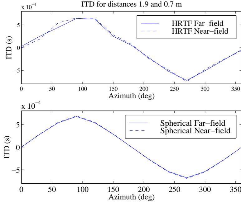
Figure 5.8: ITD plots in far-field and near-field for HRTFs measured on human subjects (top graph, mean of 9 subject ITDs) and a spherical head model (bottom graph).
