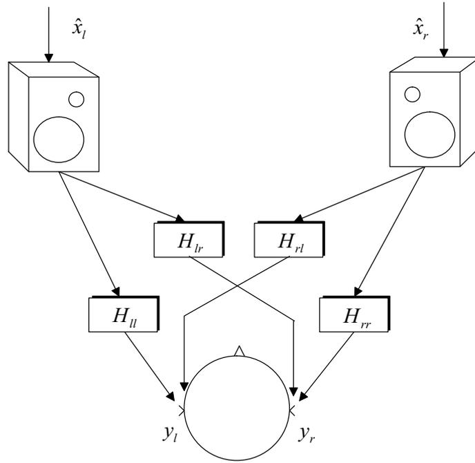
Figure 6.1: Loudspeaker-to-ear transfer functions in stereophonic listening arrangement.
