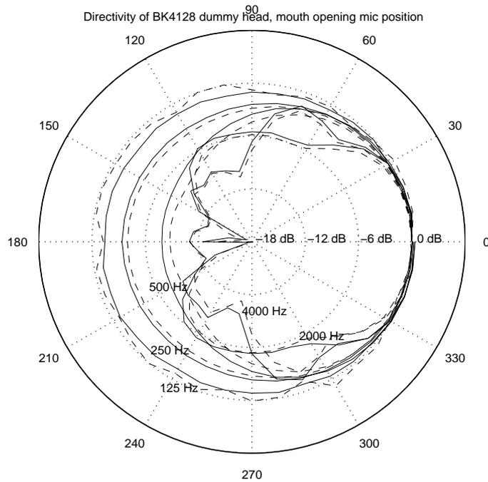
Figure 3.6: Directivity of the BK4128 dummy head using the direct method (dashed line) and the reciprocity method (solid line). The reciprocal microphone position is at the mouth transducer position (14 mm inside the mouth opening).
