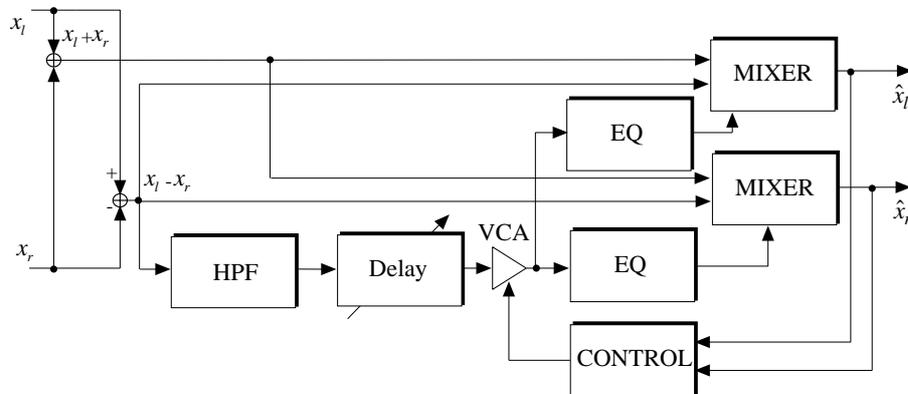
Figure 6.14: Stereo widening algorithm presented in (Desper, 1995).
