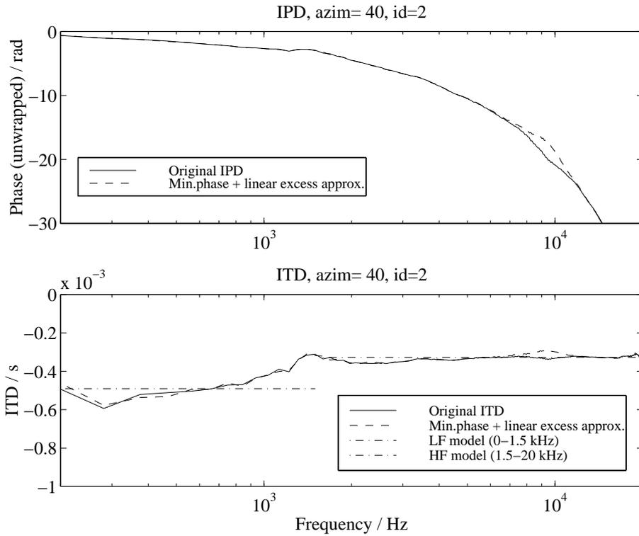
Figure 5.5: Estimation of the ITD using the minimum-phase and linear excess phase approximation method (Jot et al., 1995). Upper plot: Original IPD (solid line) and IPD approximation (dashed line). Lower plot: Original ITD (solid line), ITD approximation (dashed line), and low-frequency and high-frequency ITD models (dash-dot lines).
