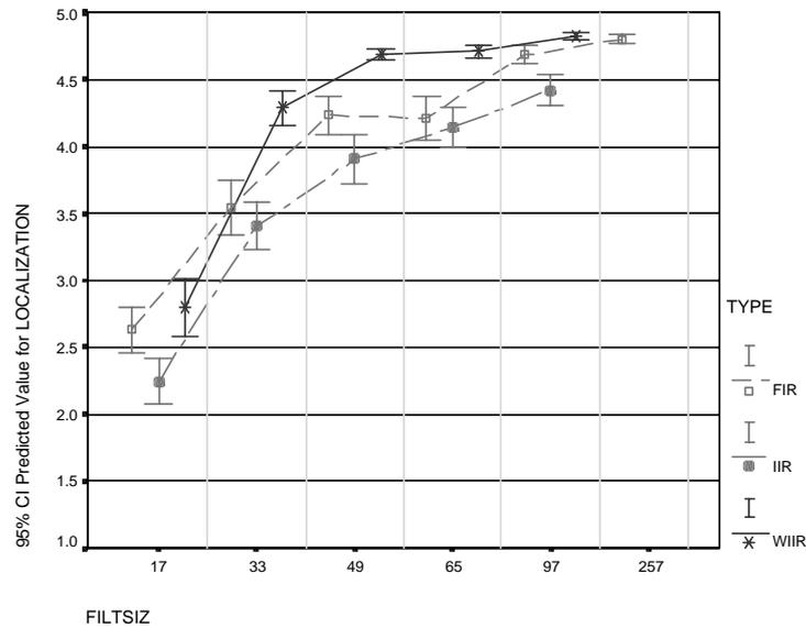
Figure 5.40: Listening test results for three filter types (FIR, IIR, WIIR). Predicted values as a function of filter type and order. Tested variable: localization (Huopaniemi et al., 1998, 1999b).
