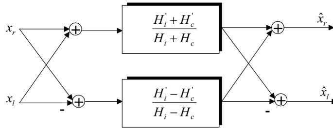
Figure 6.8: Shuffler structure for VL synthesis of two sound sources.
