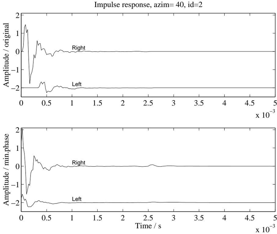
Figure 5.2: Upper plot: Mixed-phase HRIRs. Lower plot: Minimum-phase HRIRs.
