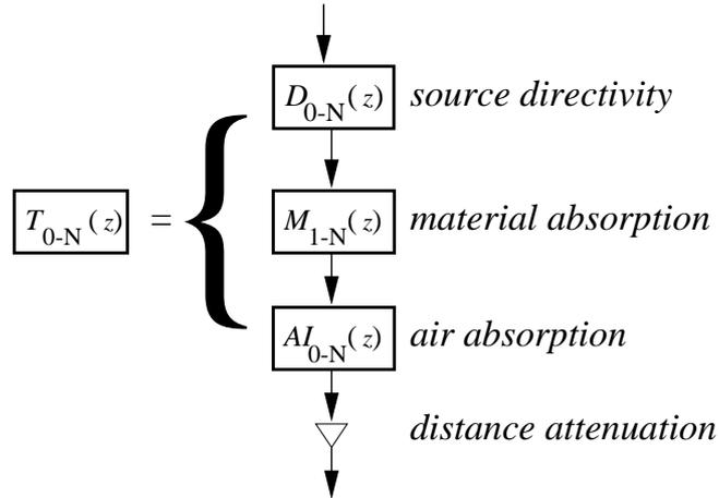
Figure 4.4: Detailed view of the real-time extended image-source modeling algorithm shown in Fig. 2.6 (page 38). The filter structure  $T_k(z)$  comprises source directivity filters  $D_k(z)$ , material absorption filters  $M_k(z)$ , air absorption filter  $AI_k(z)$ , and a gain factor for the  $1/r$  attenuation law (Savioja et al., 1999).
