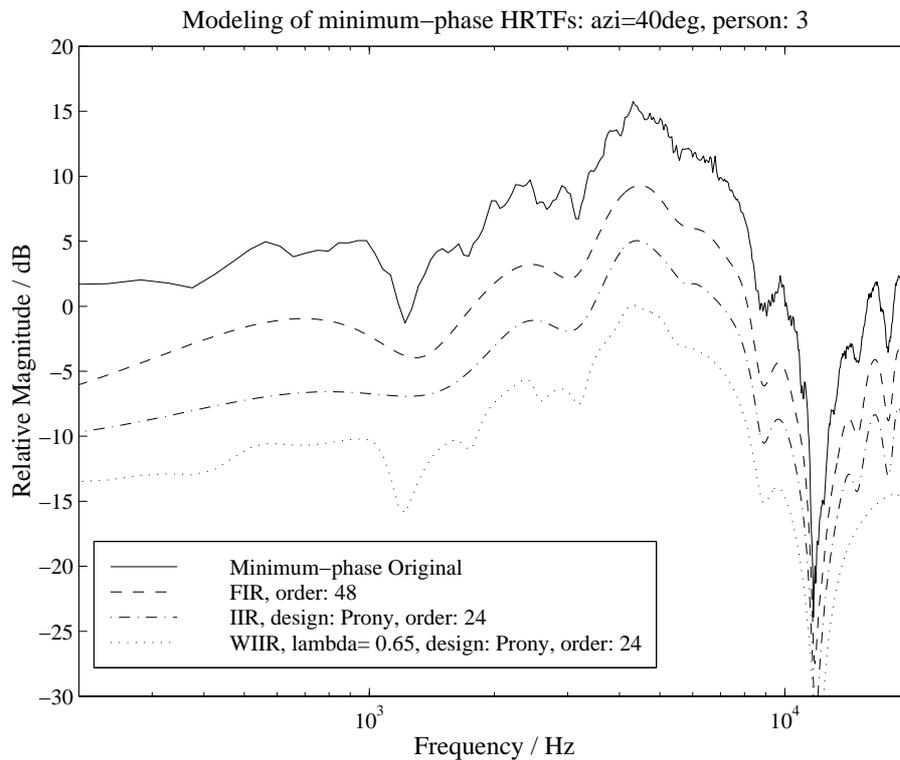
Figure 5.31: HRTF magnitude response and different filter approximations. Right ear, azimuth angle  $40^\circ$ , person 3 (Huopaniemi et al., 1998, 1999b).
