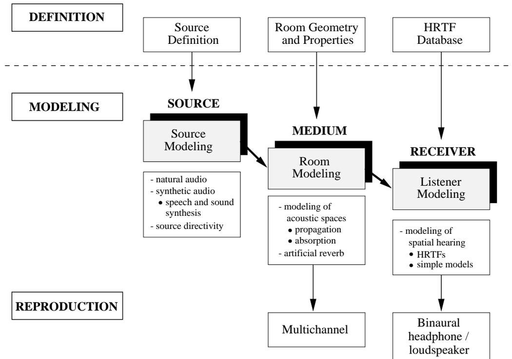
Figure 2.1: Modeling concept of virtual acoustics (Huopaniemi, 1997; Savioja et al., 1999).
