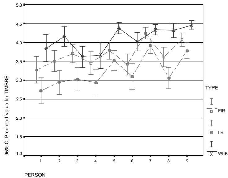
Figure 5.39: Listening test results for three filter types (FIR, IIR, WIIR). Predicted values as a function of test persons. Tested variable: timbre (Huopaniemi et al., 1998, 1999b).
