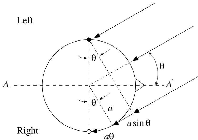
Figure 5.4: ITD approximation based on distance difference of a sound arriving at the two ears.
