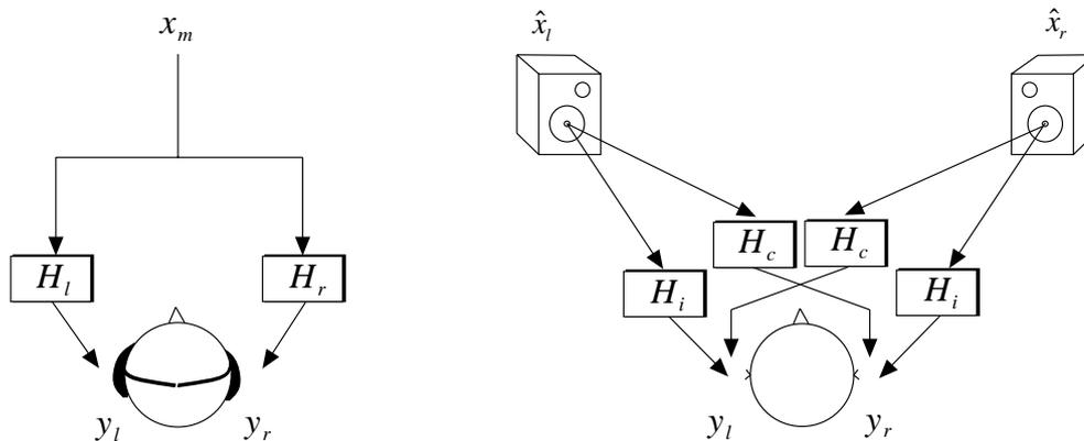
Figure 2.2: Signal flowgraph of a) binaural and b) crosstalk canceled binaural audio processing.
