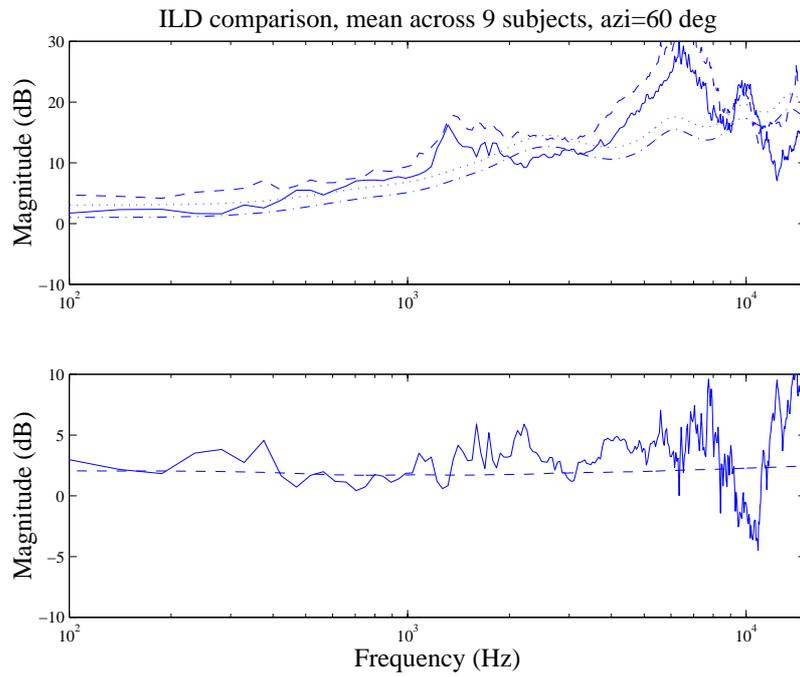
Figure 5.13: Near-field and far-field interaural level differences at  $60^\circ$ .
