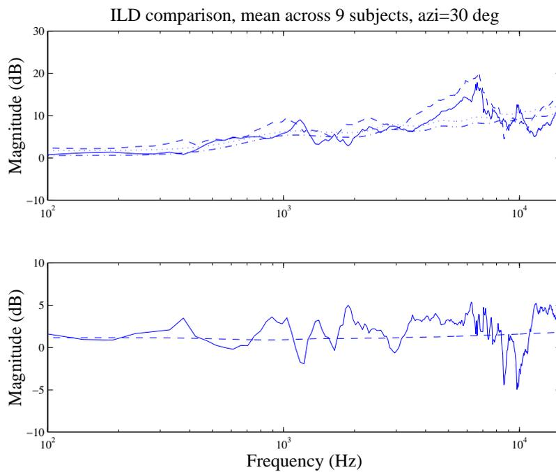
Figure 5.12: Near-field and far-field interaural level differences at  $30^\circ$ .
