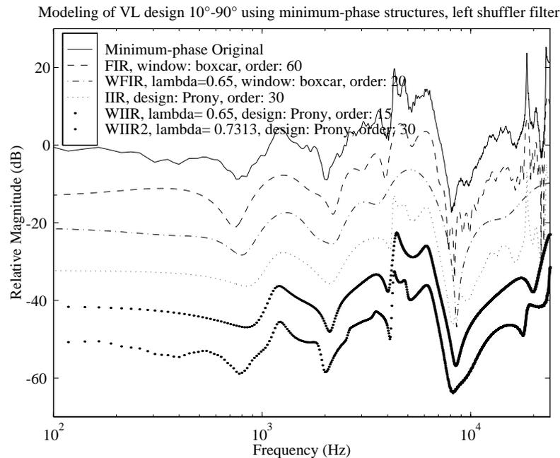
Figure 6.18: Virtual loudspeaker filter design for  $10^\circ - 90^\circ$  using FIR, IIR, WFIR, and WIIR filters.
