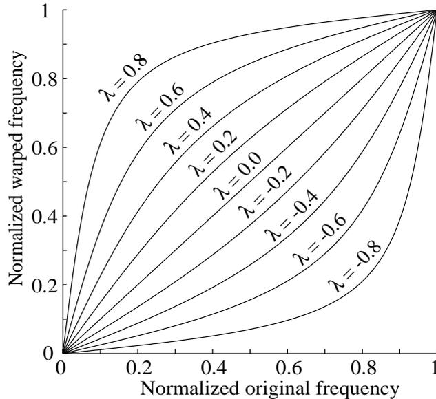
Figure 5.19: Frequency warping characteristics of the first-order allpass section  $D_1(z)$  for different values of  $\lambda$ . Frequencies are normalized to the Nyquist rate (Karjalainen et al., 1999).
