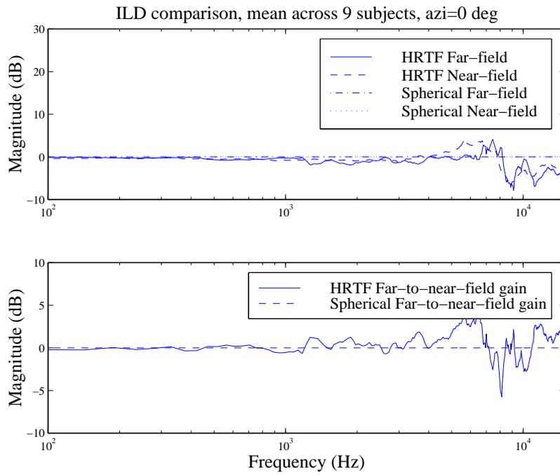
Figure 5.11: Near-field and far-field interaural level differences at  $0^\circ$ .
