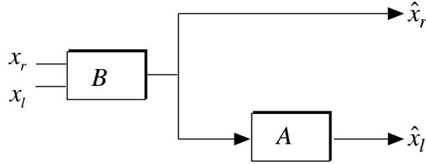
Figure 6.7: Spectral stereo shuffler for synthesis of one virtual loudspeaker.
