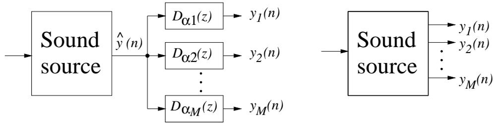
Figure 3.1: Two methods for incorporating directivity into sound source models: (a) directional filtering, (b) set of elementary sources (Karjalainen et al., 1995; Savioja et al., 1999).
