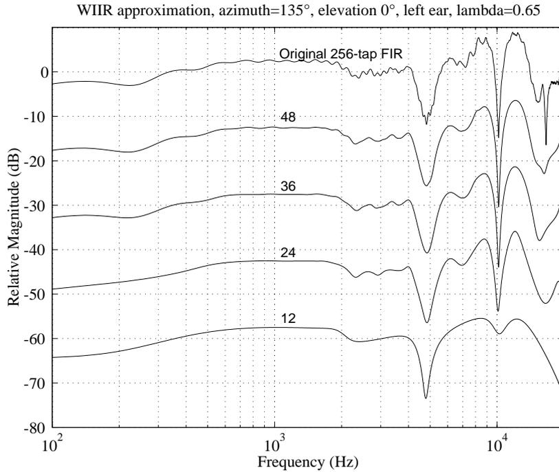
Figure 5.28: WIIR filter design of Cortex dummy head HRTFs (135° azimuth). WIIR filter orders: 12, 24, 36, 48 (Huopaniemi and Karjalainen, 1997).
