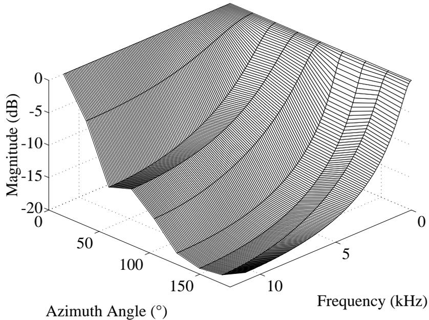
Figure 3.2: Modeling the directivity characteristics of the trumpet with first-order IIR filters. The azimuth interval of modeled responses is  $22.5^\circ$  (Karjalainen et al., 1995).
