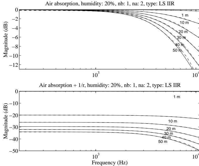
Figure 4.3: Magnitude response of air absorption filters as function of distance (1m-50m) and frequency. The continuous line represents the ideal response and the dashed is the filter response. The air humidity is chosen to be 20% and temperature 20°C. Upper plot: air absorption only. Lower plot: air absorption +  $1/r$  distance attenuation.
