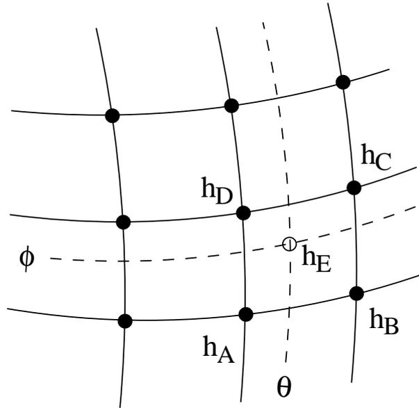
Figure 5.23: HRTF-filter coefficients corresponding to point  $h_E$  at azimuth  $\theta$  and elevation  $\phi$  are obtained by bilinear interpolation from measured data points  $h_A$ ,  $h_B$ ,  $h_C$ , and  $h_D$  (Begault, 1994; Savioja et al., 1999).
