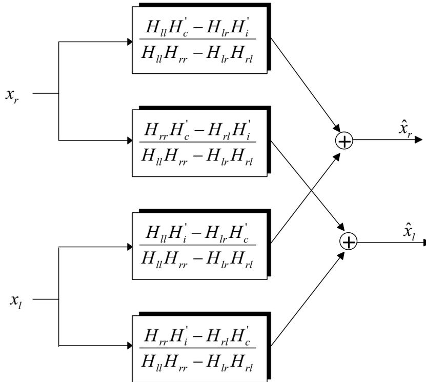
Figure 6.11: Direct structure for VL synthesis of two sound sources in asymmetrical listening.
