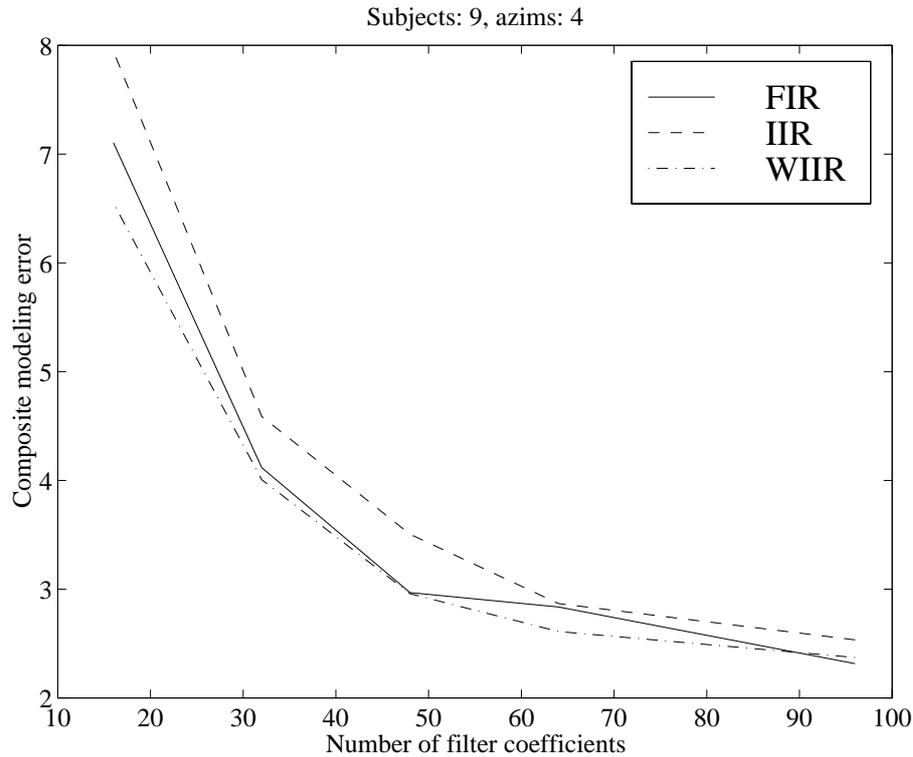
Figure 5.35: Binaural auditory model results for 9 subjects and 4 azimuth angles using three different filter design methods. The composite (L + R) loudness level spectrum error estimate was used (Huopaniemi et al., 1998, 1999b).
