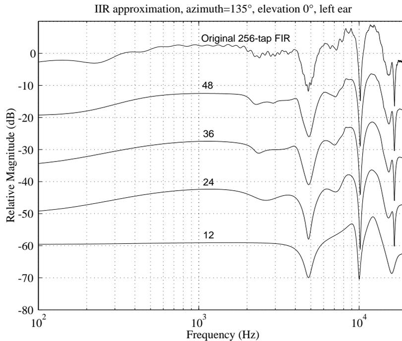
Figure 5.27: IIR filter design of Cortex dummy head HRTFs ( $135^\circ$  azimuth). IIR filter orders: 12, 24, 36, 48 (Huopaniemi and Karjalainen, 1997).
