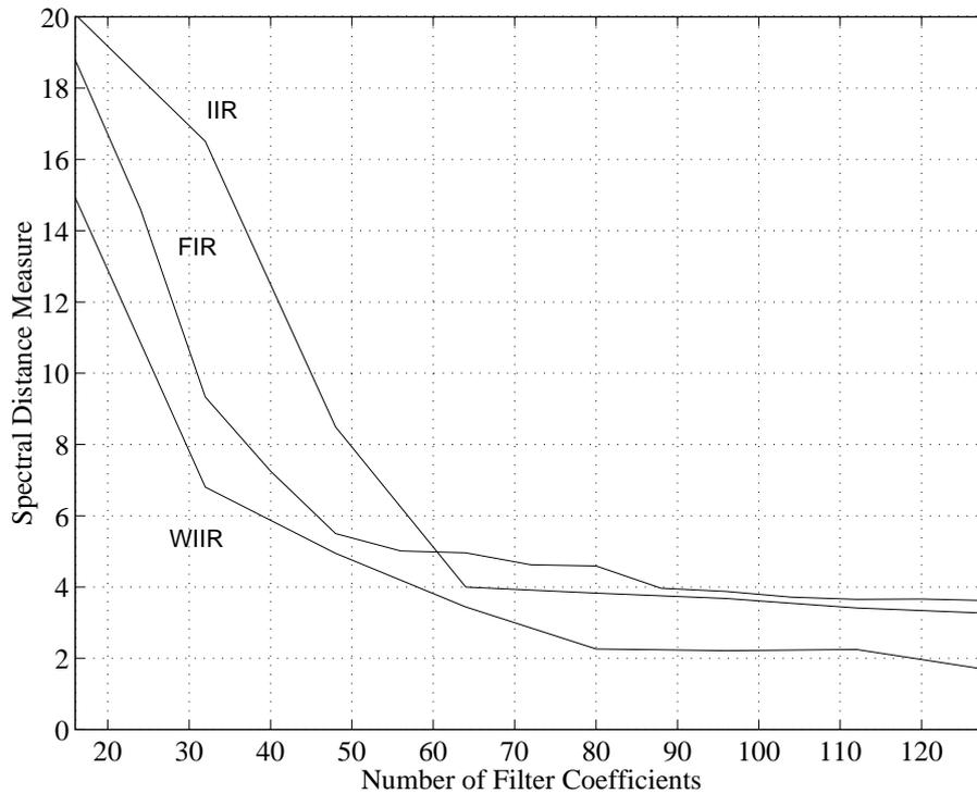
Figure 5.29: Characterization of filter design quality using a spectral distance measure as a function of the number of filter coefficients for the three filter types of the study: FIR, IIR, and WIIR (Huopaniemi and Karjalainen, 1997).
