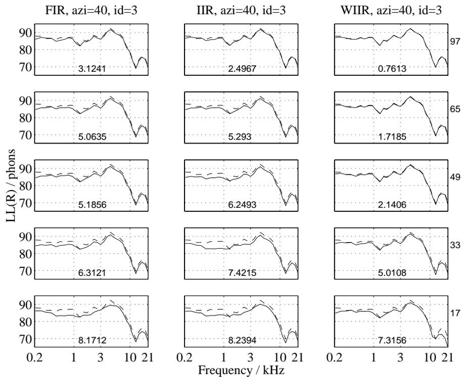
Figure 5.33: Binaural auditory model evaluation of filter design quality. Right ear, azimuth angle  $40^\circ$ , person 3. Solid line: filter approximation, dashed line: reference (Huopaniemi et al., 1998, 1999b).
