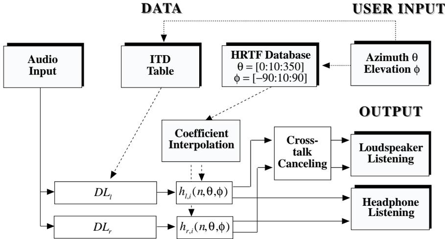
Figure 5.1: General implementation framework of dynamic 3-D sound using non-recursive filters. HRTF modeling is carried out using pure delays to represent the ITD ( $DL_l$  and  $DL_r$ ), and minimum-phase reconstructed interpolated HRIRs ( $h_{l,i}(n)$  and  $h_{r,i}(n)$ ).
