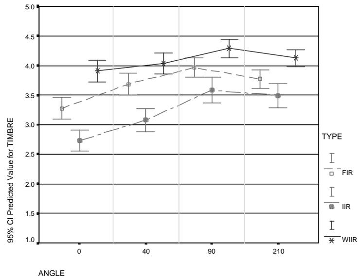
Figure 5.43: Listening test results for three filter types (FIR, IIR, WIIR). Predicted values as a function of presentation angle. Tested variable: timbre (Huopaniemi et al., 1998, 1999b).
