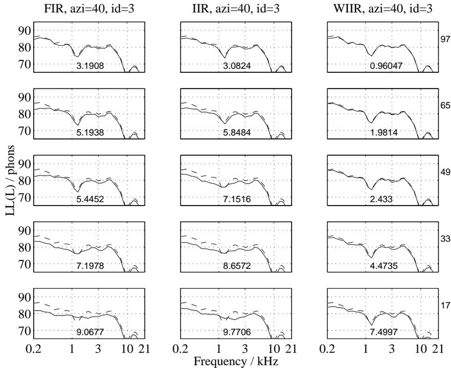
Figure 5.32: Binaural auditory model evaluation of filter design quality. Left ear, azimuth angle  $40^\circ$ , person 3. Solid line: filter approximation, dashed line: reference (Huopaniemi et al., 1998, 1999b). The RMS error is shown on each graph, and the corresponding number of filter coefficients is given on the right side of the figure.
