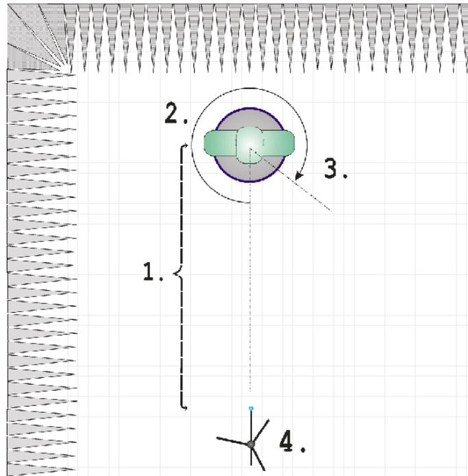
Figure 3.4: Measurement installation in the anechoic chamber for the direct method. **1.** Distance to source (the mouth speaker of the dummy head): 2 meters. **2.** Azimuth angle. **3.** Rotational direction of the BK4128 dummy head placed on a turntable. **4.** Measurement microphone (Sennheiser KE 4-211-2) on stand (Huopaniemi et al., 1999a).
