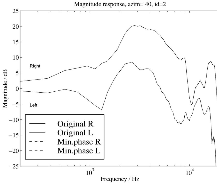
Figure 5.3: Mixed-phase and minimum-phase HRTFs (note that the mixed-phase and minimum-phase magnitude responses are equal).
