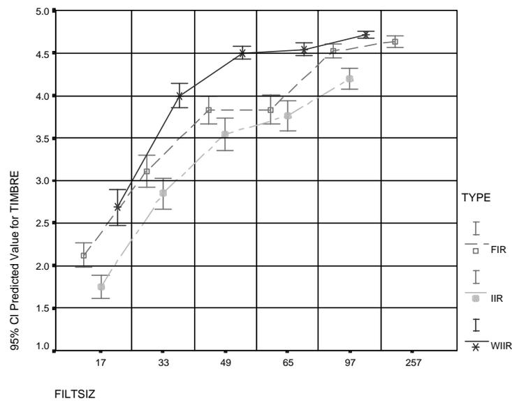
Figure 5.41: Listening test results for three filter types (FIR, IIR, WIIR). Predicted values as a function of filter type and order. Tested variable: timbre (Huopaniemi et al., 1998, 1999b).
