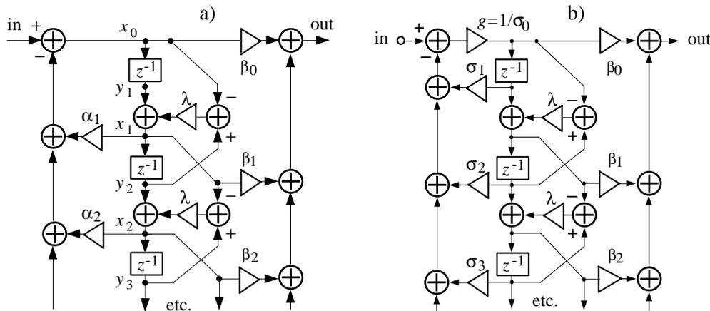
Figure 5.22: WIIR structures (Karjalainen et al., 1999). a) Unrealizable direct form of WIIR filter. b) Realizable modified implementation used in present study.
