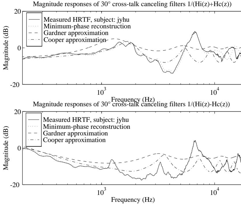
Figure 6.3: Magnitude responses of three crosstalk canceling filters for sources at  $30^\circ$  azimuth.
