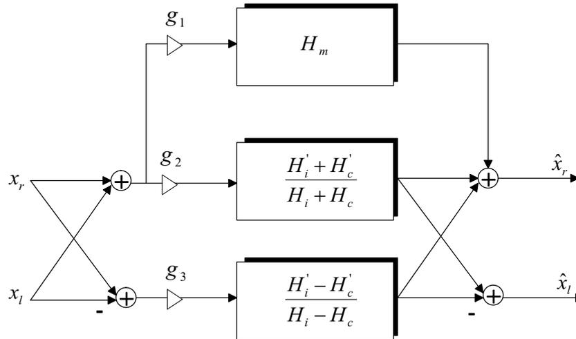
Figure 6.17: Stereo widening algorithm based on virtual loudspeaker positioning and control of the monophonic sound.
