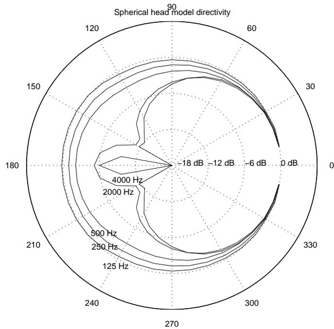
Figure 3.8: Directivity of the analytical spherical head approximation.
