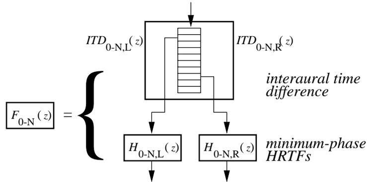
Figure 4.5: Detailed view of the real-time extended image-source modeling algorithm shown in Fig. 2.6 (page 38). The filter structure  $F_k(z)$  implements the interaural time delays  $ITD_k$  and the minimum-phase HRTFs  $H_k(z)$  (Savioja et al., 1999).
