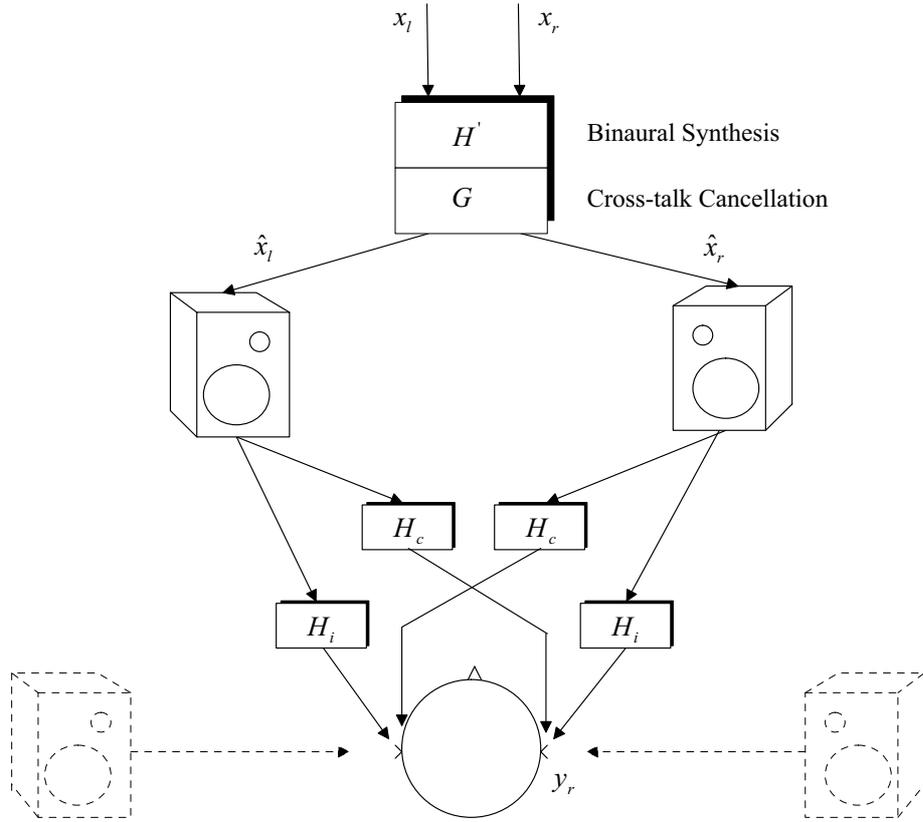
Figure 6.5: Signal transmission for cross-talk cancellation in virtual loudspeaker synthesis.
