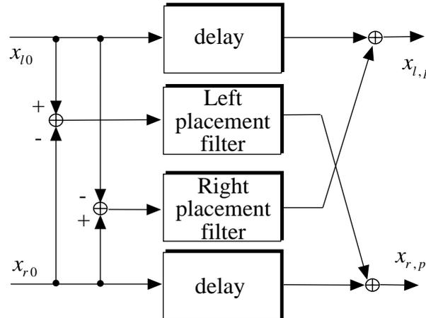
Figure 6.16: Stereo widening algorithm presented in (Lowe et al., 1995).
