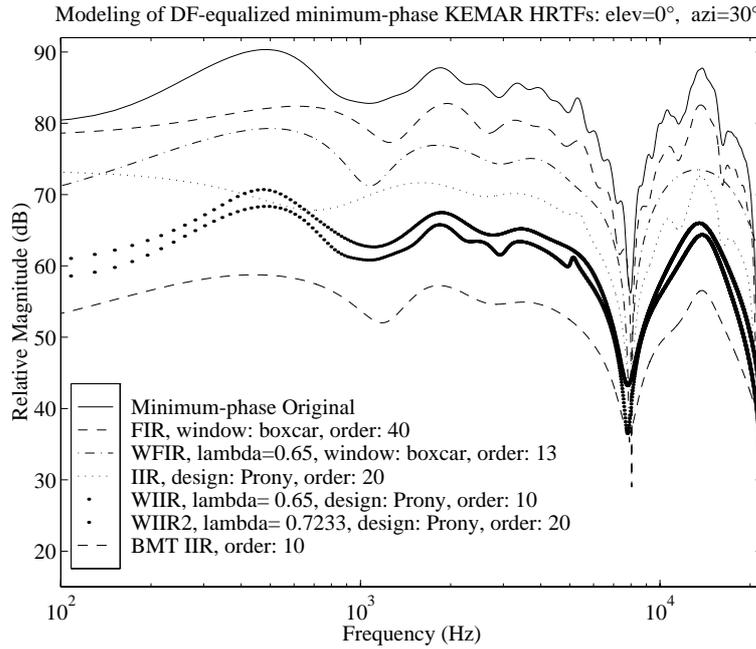
Figure 5.25: Warped filter design compared with traditional FIR and IIR designs. Kemar dummy head HRTFs were used (Huopaniemi and Karjalainen, 1996b,a).
