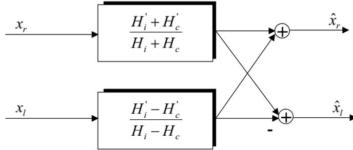
Figure 6.6: Shuffler structure for VL synthesis of one virtual source.
