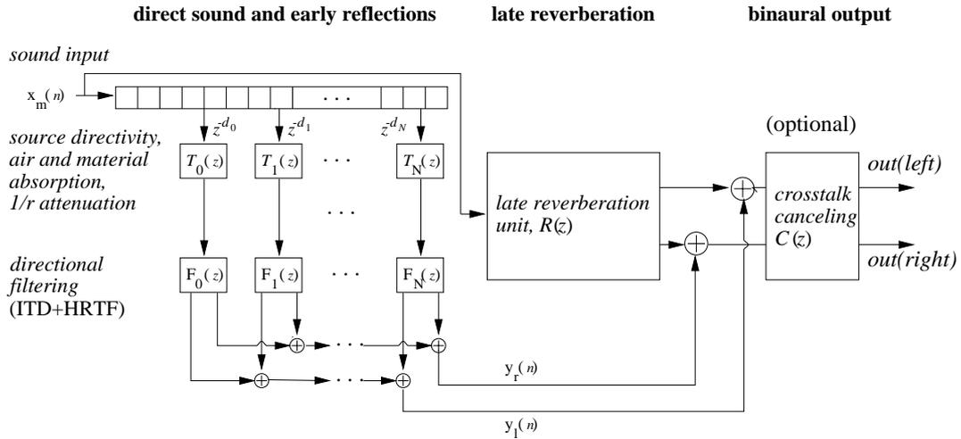
Figure 2.6: Implementation of virtual acoustics using geometrical acoustics modeling. The direct sound, early reflections and late reverberation are processed separately, enabling a fully parametric implementation.
