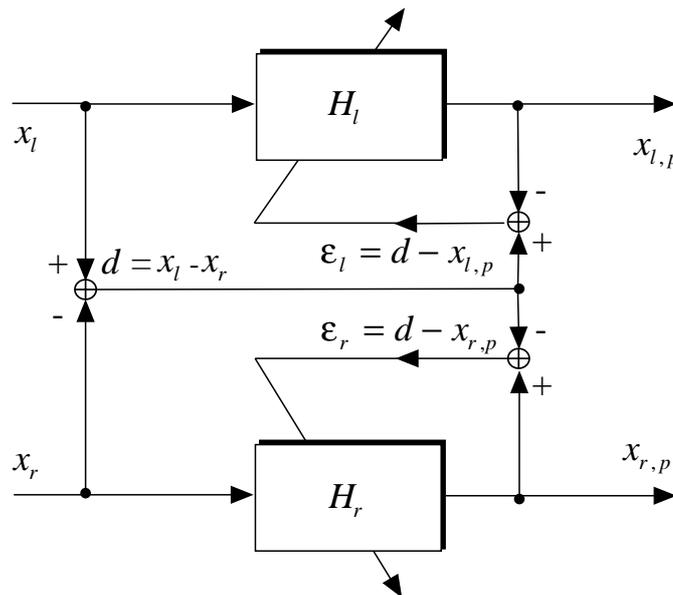
Figure 6.15: Stereo widening algorithm presented in (Maher et al., 1996).
