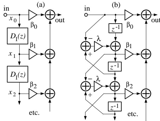
Figure 5.21: WFIR structures (Karjalainen et al., 1999). a) Principle of warped FIR filter. b) Implementation used in present study (Karjalainen et al., 1997a).
