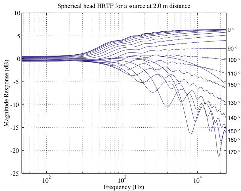
Figure 5.10: HRTFs computed from a Rayleigh diffraction model (Duda and Martens, 1998). Source distance: 2.0m.
