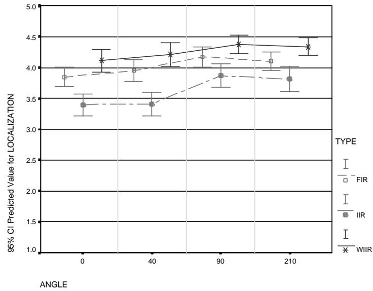
Figure 5.42: Listening test results for three filter types (FIR, IIR, WIIR). Predicted values as a function of presentation angle. Tested variable: localization (Huopaniemi et al., 1998, 1999b).
