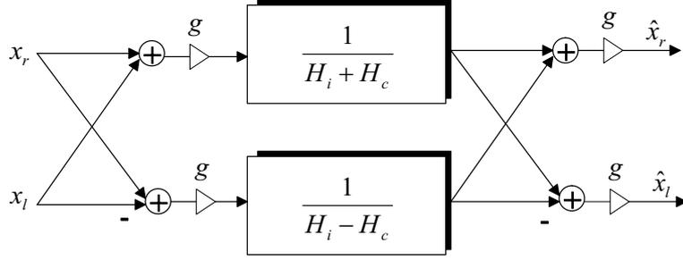
Figure 6.2: Shuffler implementation of cross-talk canceling filters in a symmetric listening arrangement.
