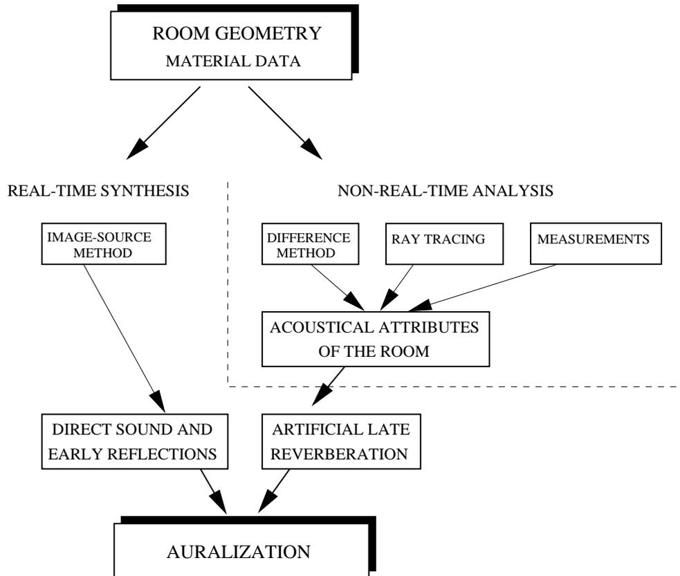
Figure 2.5: Computational room acoustic rendering methods used in the DIVA system. The model is a combination of a real-time image-source method and artificial reverberation which is parametrized according to room acoustical parameters obtained by simulation or measurements (Savioja et al., 1999).
