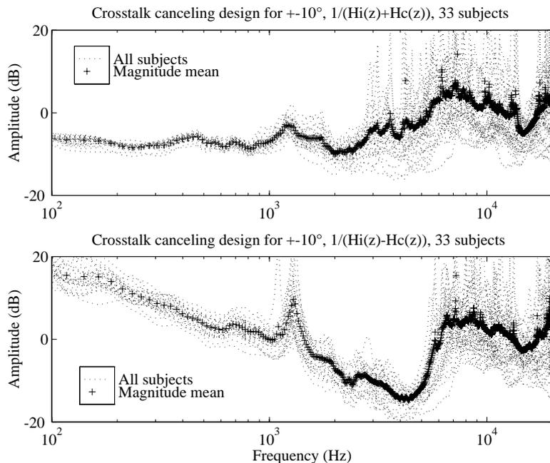
Figure 6.19: Crosstalk canceling magnitude responses for loudspeakers placed at  $\pm 10^\circ$  azimuth based on 33 human subject HRTFs (shown as dotted lines). The line marked with (+) represents a calculated mean of the magnitude responses.
