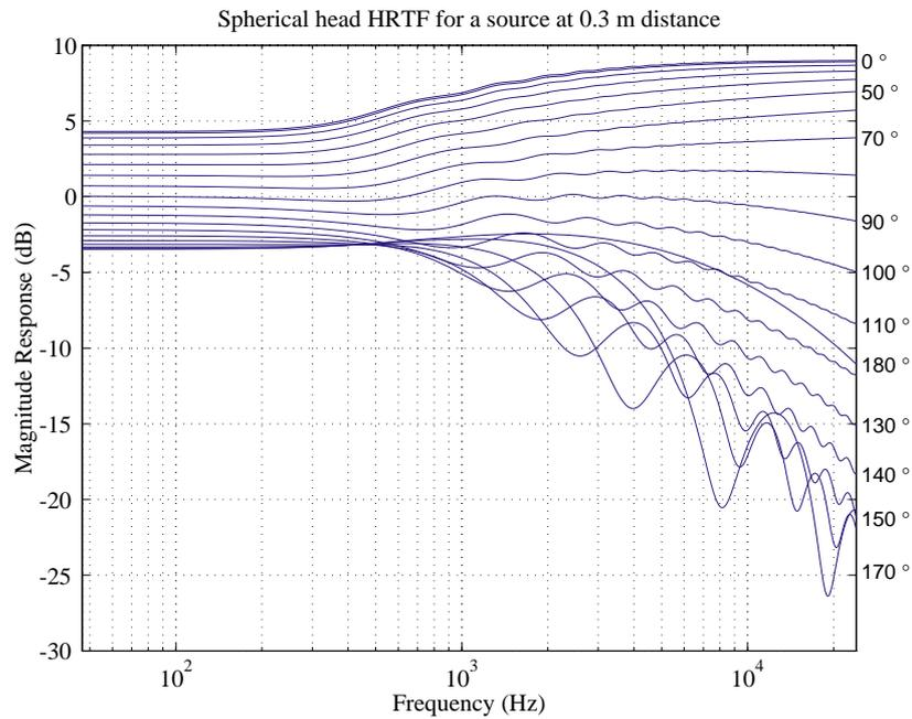
Figure 5.9: HRTFs computed from a Rayleigh diffraction model (Duda and Martens, 1998). Source distance: 0.3m.
