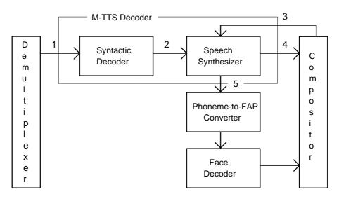
Fig. 7.1. MPEG-4 Audio TTS decoder architecture.
