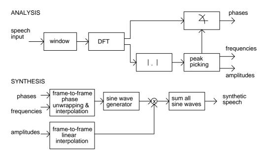
Fig. 5.6. Sinusoidal analysis / synthesis system (Macon 1996).
