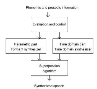
Fig. 5.7. Basic idea of the hybrid synthesis system
