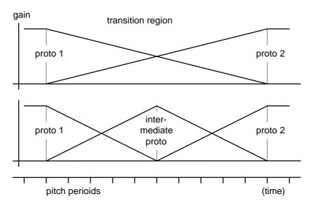
Fig. 5.5. Linear amplitude based interpolation (Lukaszewicz et al. 1997).
