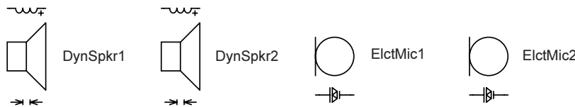
Figure 5.8: Dynamic loudspeakers, electret microphones (omnidirectional and pressure gradient type).
